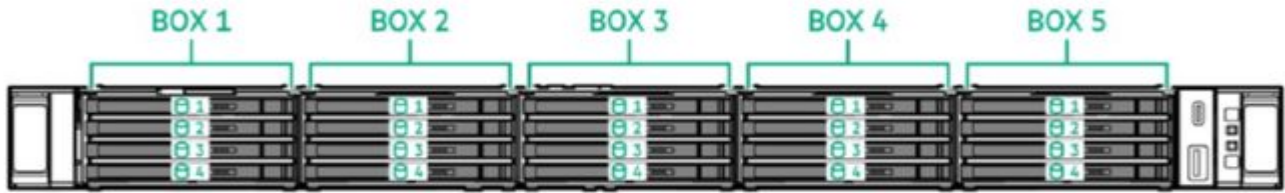
20 E3.S device box & bay numbering (P72176-B21)
